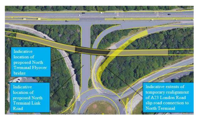
Figure 21: Proposed New Flyover, NT link road and A23 Slip Road connection
