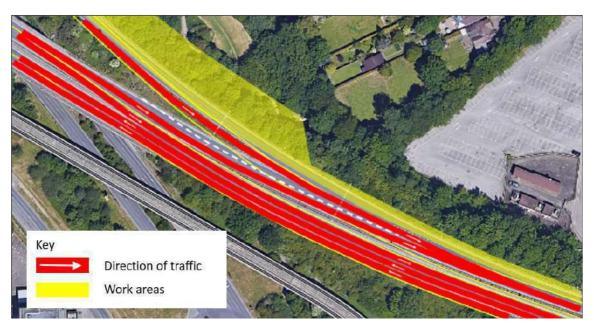
Figure 18: Detail at Airport Way Eastbound Contraflow in Stage W4
